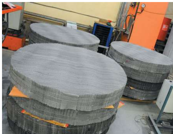
Fig. 1. Mesh packing "Chevron". JSC "Intarex" production facility
