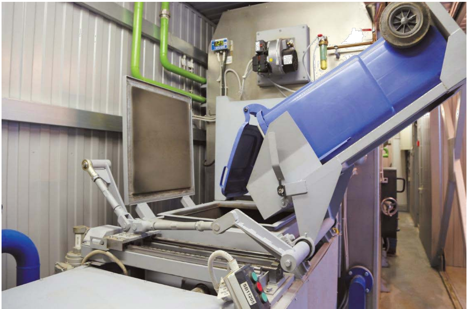
Incineration plant KTO-50.K40. Automatic loading system excludes service personnel contacts with hazardous medical waste
