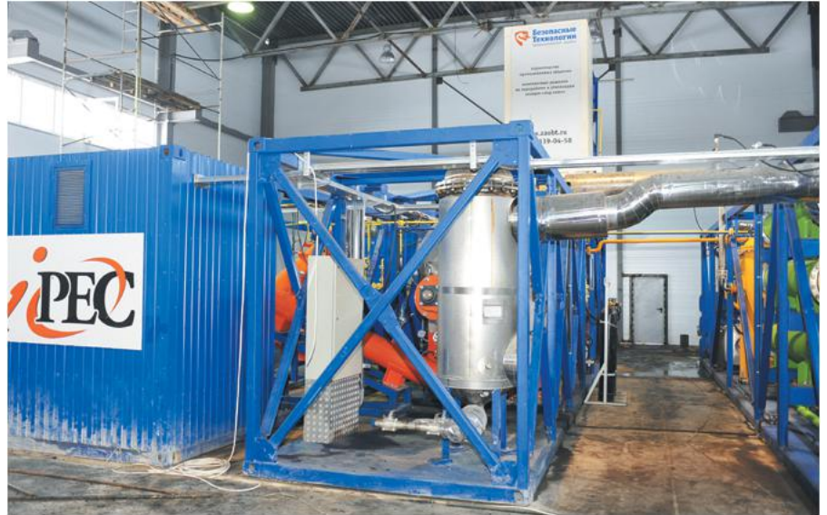
Thermal Decomposition Plant TDP-2-800 for used tires and rubber processing, Smolensk region
